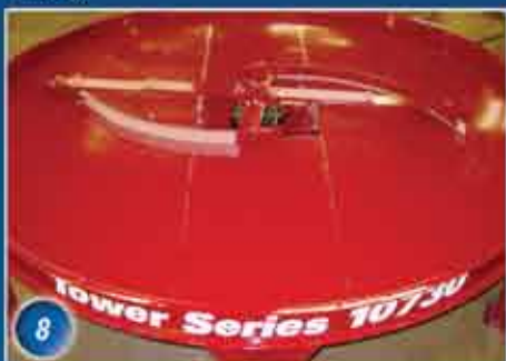
8 AC Inverter driven sweep arms control the unload rate of the dryer. No restricted flow of grain, no plugging. With every sweep arm pass, stainless steel grain discharge deck is cleaned.
