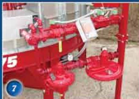
7 Gas manifold with microprocessor controlled electronic gas proportional valve allows complete control of plenum temperature for all grains to be dried. No matter how the outside temperature changes, a constant plenum temperature is automatically maintained. Digital readout on microprocessor displays plenum temperature and set point during dryer operation.
