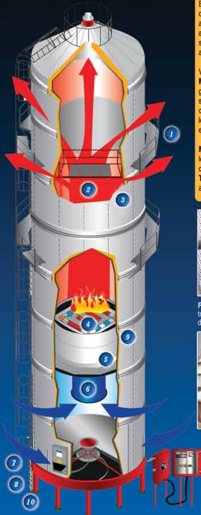
8 AC Inverter driven sweep arms control the unload rate of the dryer. No restricted flow of grain, no plugging. With every sweep arm pass, stainless steel grain discharge deck is cleaned.
